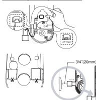
Install the door side magnetic sensor.
