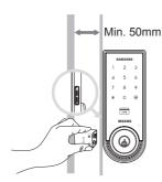
Please, be aware of that there has be more than 50mm gap between the door frame and the external power contact to place the 9V battery for temporary access.
